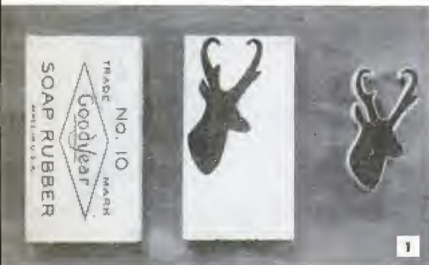
Pattern for plastic-inlay design is traced on soap-rubber eraser and cut out, as above. Sides of cutout pattern must be perpendicular. Below, pattern is placed in bottom of aluminum-foil trough and rubber-mold material is poured over it
